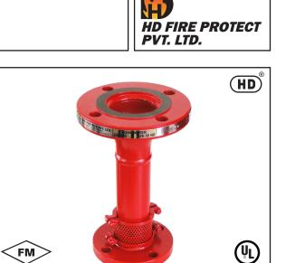
The air is drawn into the foam solution through holes located on the foam maker covered with stainless steel screen to exclude nesting birds and insects. The aerated foam is directed into the pourer for the gentle application of the expanded foam. The pourers are available in different models.\*
